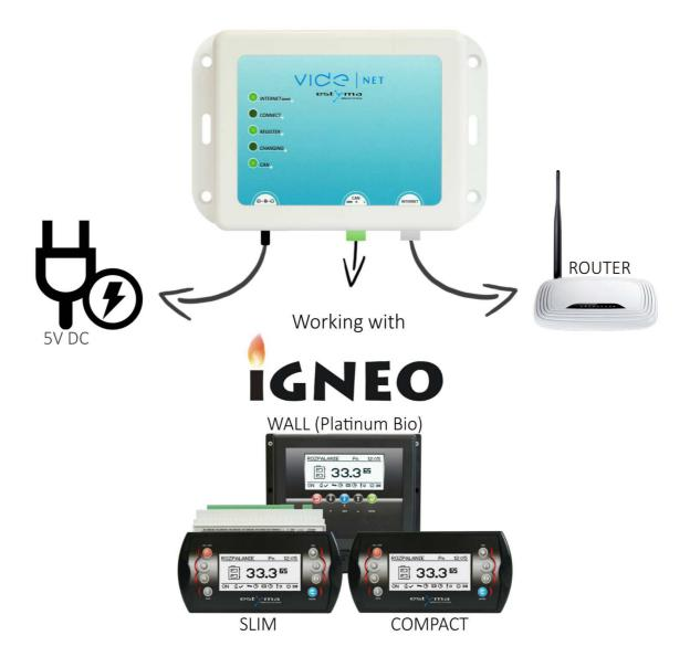
The router must have the DHCP so that the equipment can establish Internet connection.
